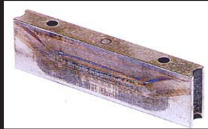
Figure 6. Impact of poor air release properties of an oil T6H20-C hybrid pump.
