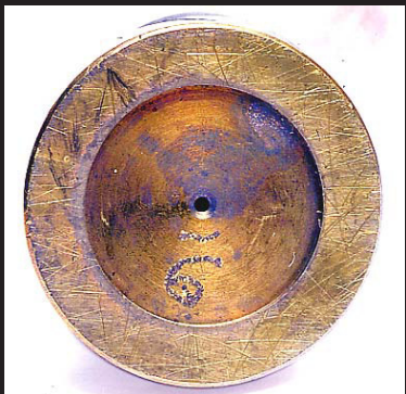
Figure 1. Scratches on a piston pump caused by particulates in the oil.
