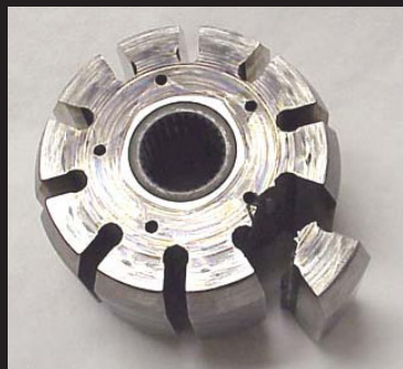
Figure 2. Lubricant-related pump failure.
