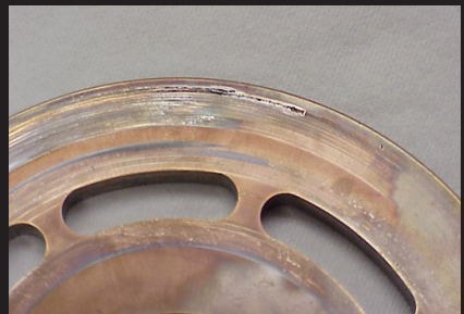
Figure 6. Impact of poor air release properties of an oil T6H20-C hybrid pump.
